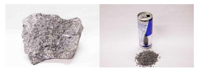
The High Energy Briquette (HEB) is designed to contain a gross energy of over 5.5 MWh/t HEB. This energy is the exothermic energy derived when the various metallic components in the HEB either oxidize or reduce components in the metallurgical system they are added to, for example:
