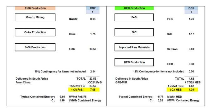
HEB Production produces only 12 % of the Carbon Footprint of FeSi75 Production.
